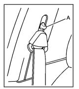
To move it down, push down the release button (A) and move the height adjuster to the desired position. You can move the height adjuster up by pushing the release button up.
